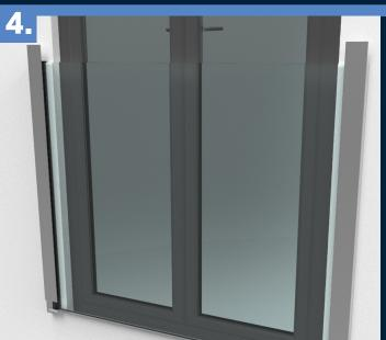
Using two people, move the glass into position so it is resting on top of the support block on both sides. With the cladding raised above the support block, hook it into position and slide down so the 2 elements are aligned.
