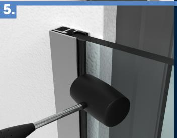
Using a rubber mallet, push the bead into the channel. This will secure the glass in place.
